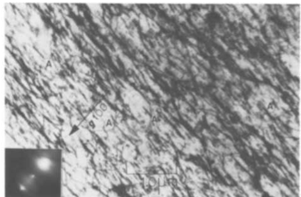
Figure 5 TEM of MgO single crystal cycled at 470°C. Higher magnification micrograph of Fig. 4.
